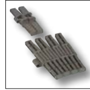
LBP 882M Sideflexing Magnetic Heavy duty single hinge Pitch 1 ½" (38,1 mm) Thickness 4,8 mm (0.189") Hinge 57 mm (2.244")
