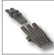
LBP 882T Sideflexing TAB Heavy duty single hinge Pitch 1 ½" (38,1 mm) Thickness 4,8 mm (0.189") Hinge 57 mm (2.244")
